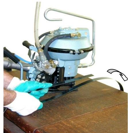
2. Grip with left hand the compressed air motor (**L**) and push the clamp lever (**K**) with the thumb (Strap gripper (**B**) open). Insert with right hand lower strap between base plate (**E**) and rocker (**C**) until it has reached the stopper. The lower strap must extend slightly (approx. **5 cm**) out of the tool. Then release the clamp lever (strap gripper (**B**) closed) so that the lower strap is fixed in its position.
