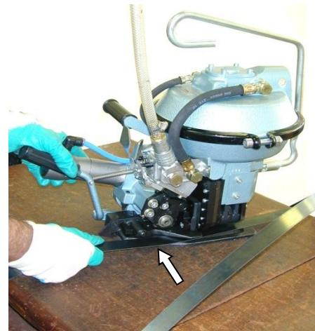
3. Grip with left hand the handle (**I**). Insert with right hand the upper strap between rocker (**C**) and transport wheel (**M**). The strap guide catch (**D**) snaps in. Keep the strap loop small by manual pre-tensioning (to avoid unnecessarily long tensioning).
