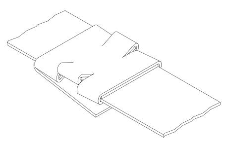
Sharp edged or misformed joints which do not appear as shown have to be taken away from the load immediately. The tensile strength of these joints is insufficient and they could cause serious injury. Having faulty joints proceed as follows:
