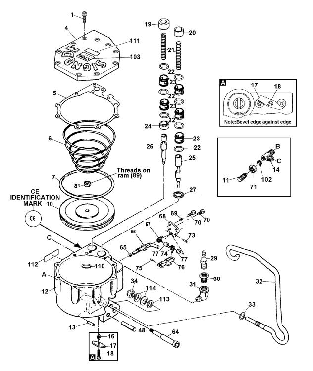
\* Apply one drop of Loctite #242 or equivalent to cleaned parts. Allow 12 hours to set, if possible. Do not apply to small screws or close moving parts as the fluid spreads easily.
