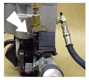
5. Press down on the operating lever once again. Air will be routed to the sealing mechanism to notch the seal/strap, cut-off the TOP STRAP and raise the feedwheel to allow the tool to be removed from the completed tie.
